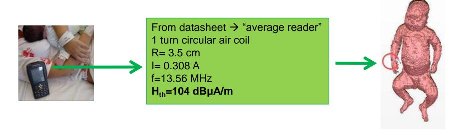
Tag → passive element, identified according to the reader technical specifications [circular ring of copper Rext=0.15 cm Rint=0.13 cm]
