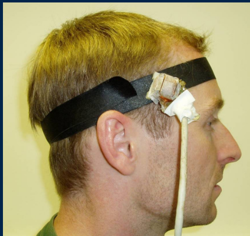
dB/dt meter based on orthogonal coils
