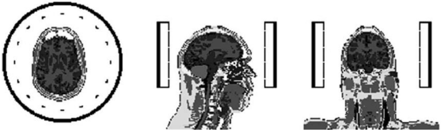
Figure 1 Coil and head model geometry on the axial, sagittal, and coronal planes passing through the coil center. Figures with greater detail have been published previously (6).
